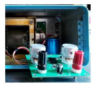
This photo was taken from the front before the new front panel was completed to illustrate how things will fit into place. The image shows the main board which will be attached directly to the front panel. Behind that is the chassis mounted reservoir capacitor and behind that, the driver board is just visible mounted on the back panel and the transformer needs no introduction of course.
