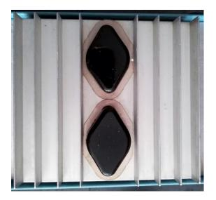
This image shows the power transistors mounted on the common heatsink using insulation kits.
