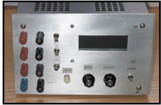
Photo 4 —To the right of the output Johnson posts are the switches that set the polarity of the floating supplies—as well as the switch that disconnects all power supply outputs—while leaving the unit still powered up.
