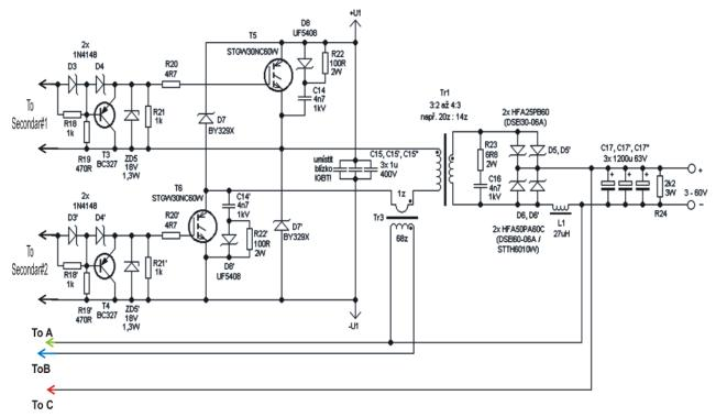
+U1 and -U1 may be derived from mains 220V input after appropriate rectification and filtration
