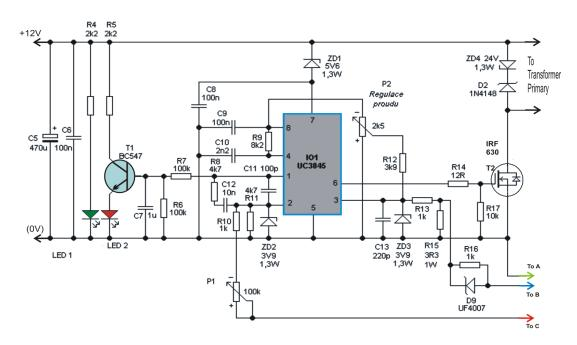
12V input supply may be acquired from an ATX power supply
