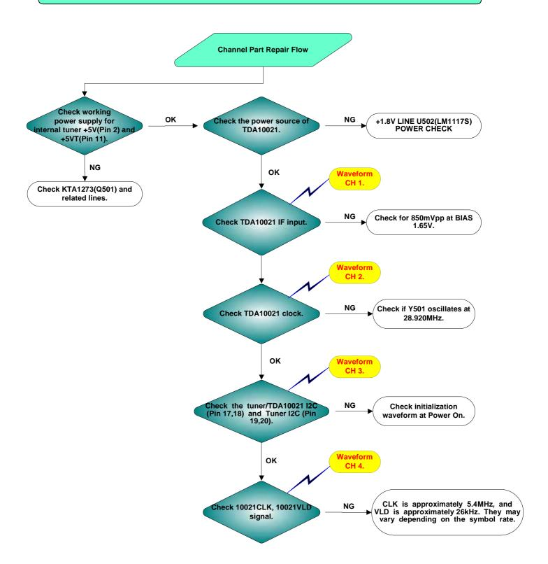
All parts including power source/CPU are working normally, but channels cannot be locked.
