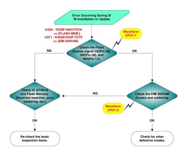
All parts including power source/CPU are working normally, but channels cannot be locked. a. Channel Part Repair Flow
