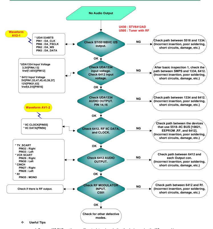
Because I2C BUS continues polling, to determine whether the devices using the I2C are working properly, check the waveforms and messages using s/w with monitor s/w or debug.
