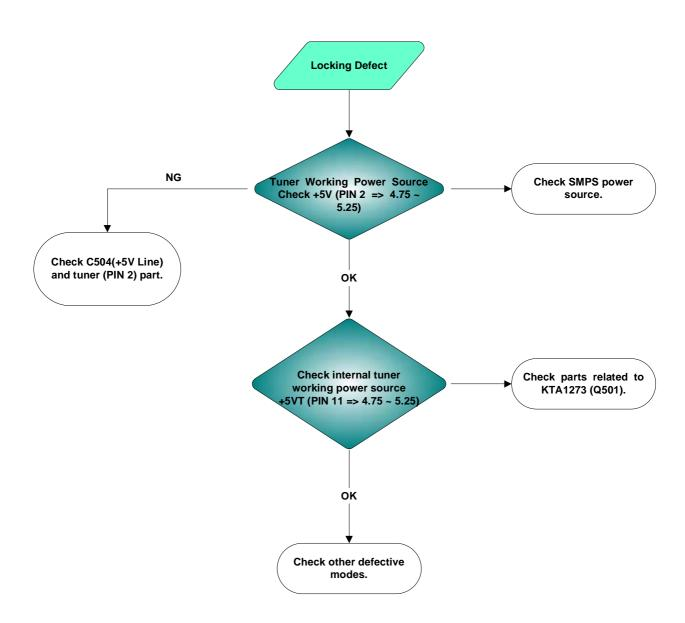
All parts including power source/CPU are working normally, but channels cannot be locked.
