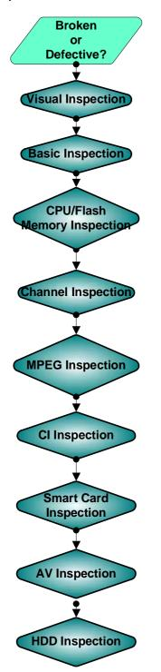
Check assembly of the set, condition of connectors, condition of the PCB, for poor soldering or short circuiting of parts, and for visual defects, and take appropriate measures.
