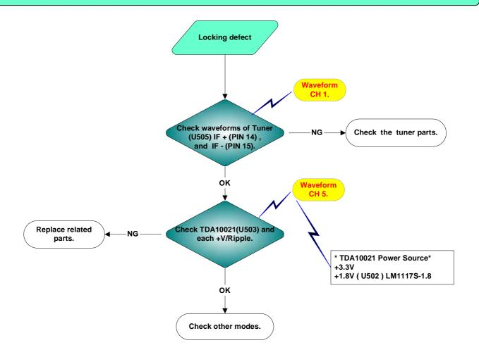
All parts including power source/CPU are working normally, but channels cannot be locked.
