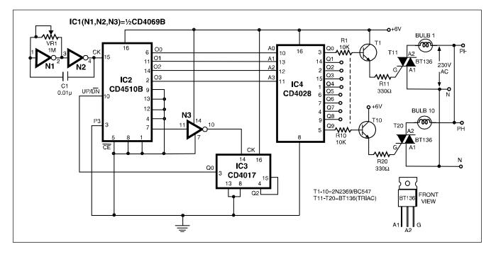
This terminal count output from pin 7, after inversion by gate N3, is connected to clock pin 14 of decade counter IC3 (CD4017) which is configured here as a toggle flip-flop by returning its Q2 output at pin 4 to reset pin 15. Thus output at pin 3 of IC3 goes to logic 1 and logic 0 state alternately at each terminal count of IC2.
