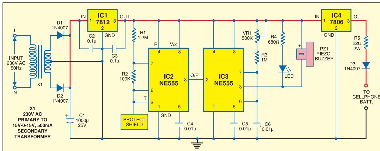
pacitor C1. Regulator IC 7812 (IC1) along with noise filter capacitors C2 and C3 provides regulated power sup-
