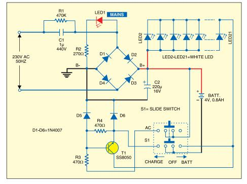
sections. The power supply section takes power from 230V AC mains supply without using a transformer. Capacitor C1 is used as an AC voltage dropper—a well-known transformerless solution. This helps to make the circuit compact without generating heat, as capacitor C1 dissipates negligible power. Capacitor C1 also protects against fluctuations in mains.
