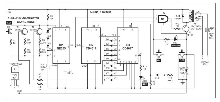
when it sounds after 30 minutes to indicate that the lunch break is over. When the last period is over, LED2 glows to indicate that the bell circuit should now be switched off manually.
