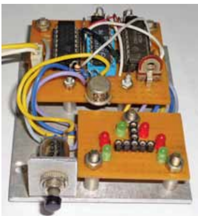
Fig. 2: Author's prototype of bipolar transistor tester
