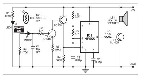
and increases the 'on' time of alarm. The higher the value of capacitor C1, the higher the forward voltage applied to the base of transistor T1 (BC548).
