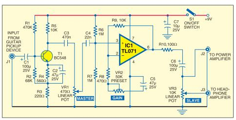
Fig. 2: Guitar preamplifier circuit
