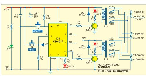
and straightforward. Whenever 12V DC is applied to the circuit, power-on LED1 glows. Now reset the decade counter by momentarily pressing switch S2 to make Q0 output of IC1 high. LED2 glows to indicate that the circuit is ready to work.
