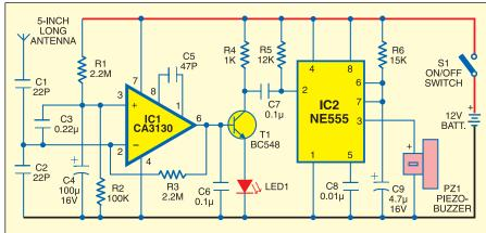
The circuit can detect both the incoming and outgoing calls, SMS and video transmission even if the mobile phone is kept in the silent mode. The moment the bug detects RF transmission signal from an activated mobile phone, it starts sounding a beep alarm and the LED blinks. The alarm continues until the signal transmission ceases.
