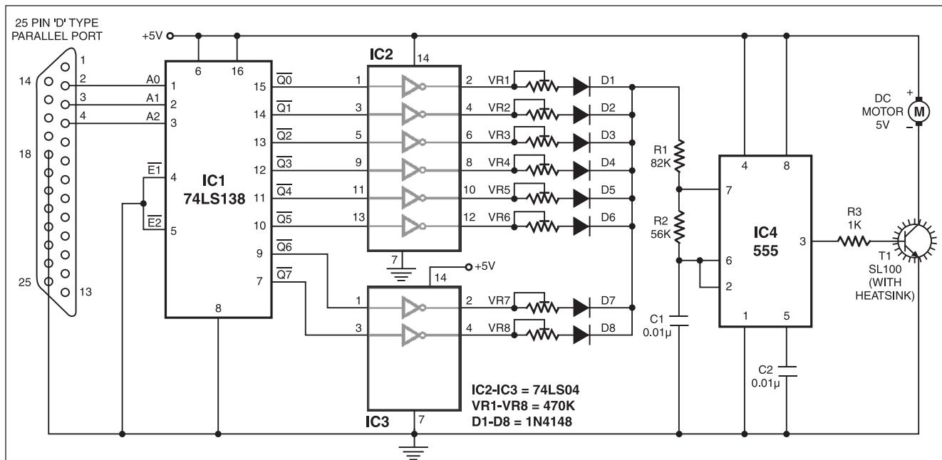
circuit consists of 1-of-8 decoder IC 74LS138 (IC1), hex inverter ICs 74LS04 (IC2 and IC3), resistor networks, timer IC 555 (IC4) and motor driver transistor SL100 (T1). The decoder IC accepts binary weighted inputs A0, A1 and A2 at pins 1, 2 and 3, respectively. With active-low enable input pins 4 and 5 of the decoder grounded, it provides eight mutually exclusive active-low outputs (Q0 through Q7). These outputs are inverted by hex inverters IC2 and IC3.
