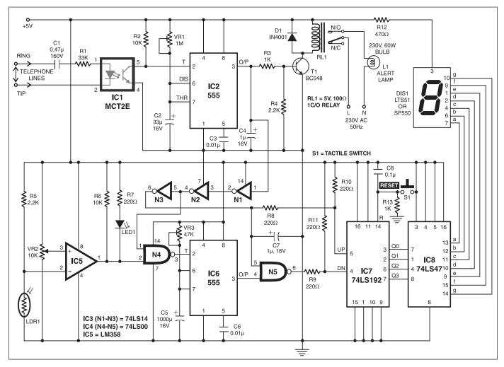
preferably using your mobile phone. The ring is detected by the given circuit and the watchman is also given a visual alert signal by a glowing lamp. The lamp remains 'on' for a duration of nearly 60 seconds soon after the ringtone. The watchman is given number of times the watchman failed to register his presence. The mobile phone records the called number and call time, and it can be used with the displayed count to get the timing details.
