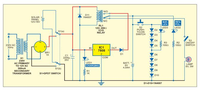
power grid. These systems are nonpolluting, don't deplete the natural resources and are cheap in the long run. The aim of this circuit is to demonstrate how we can utilise solar light to electrify the remote areas, i.e., how we can store the solar energy and then use it for small-scale lighting applications.
