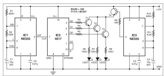
by one. In this circuit, the LEDs flash a number of times one by one.
