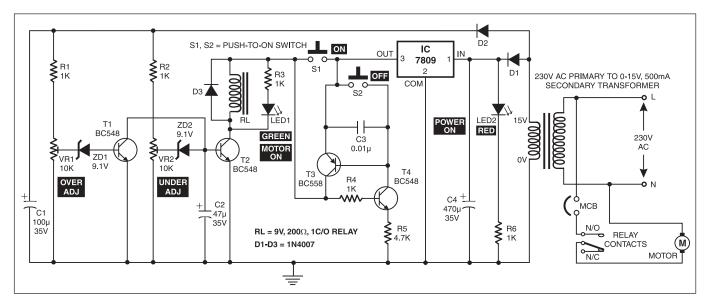
D2 rectify the AC voltage to DC. The unregulated power supply is given to the protection circuit.
