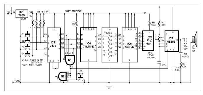
to which of the four contestants first pressed the button and locks out the remaining three entries. Simultaneously, an audio alarm and the correct decimal number display of the corresponding contestant are activated.
