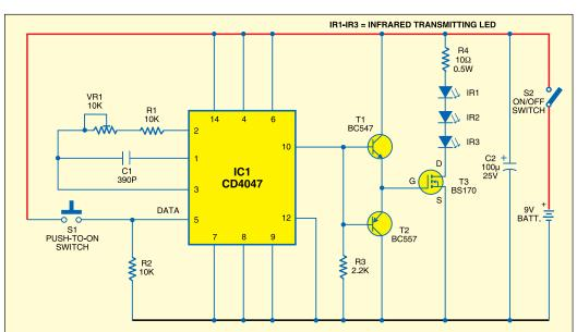
Fig. 1: Circuit of the long-range IR transmitter
