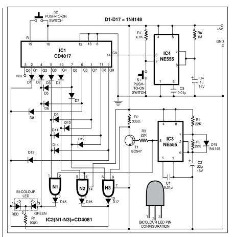
plied to pin1, it emits red light. Similarly, when positive voltage is applied to pin3, it emits green light. And when positive voltage is simultaneously applied to its pin1 and 3, it emits yellowish light.
