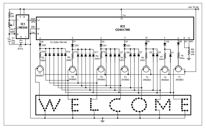
the IC ideal for use in a whole range of sequencing operations. In the circuit only one of the outputs remains high and the other outputs switch to high state successively on the arrival of each also remains lighted because of forward biasing of transistor T7 via diode D21. In a similar fashion, on the arrival of each successive pulse, the other letters of the display are also illuminated and finally
