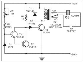
sensor D1 must be of germanium type and not silicon.
