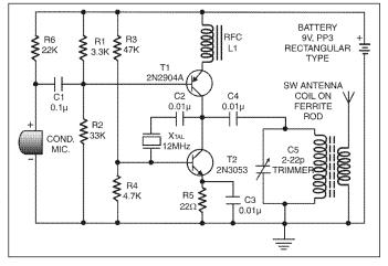
loop antenna into space in the form of electromagnetic waves. The antenna can be tuned to a particular frequency varying trimmer C5 and also by changing the length of ferrite rod into the coil.
