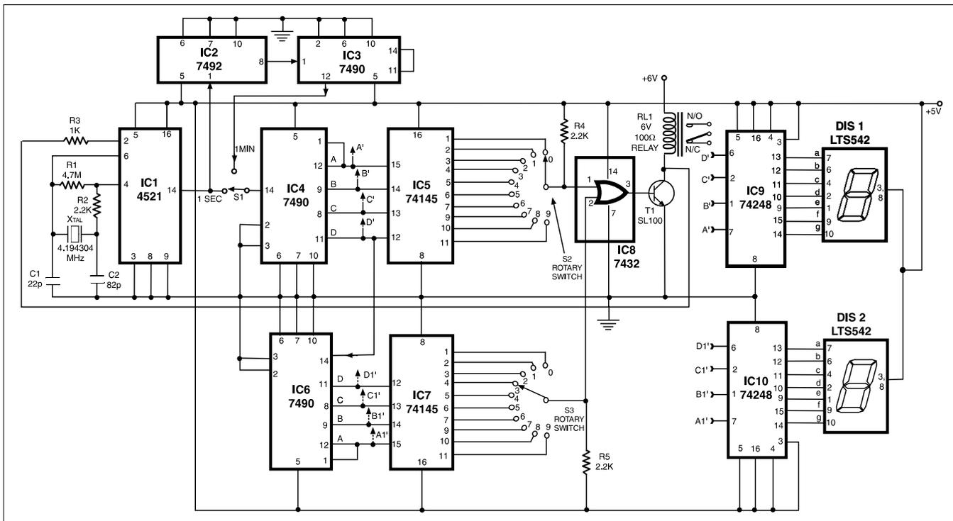
The decade counter IC4 provides binary output as it counts up the input pulses and IC5 decodes/converts them to 1-of-10 outputs (units). Similarly, the IC6-
