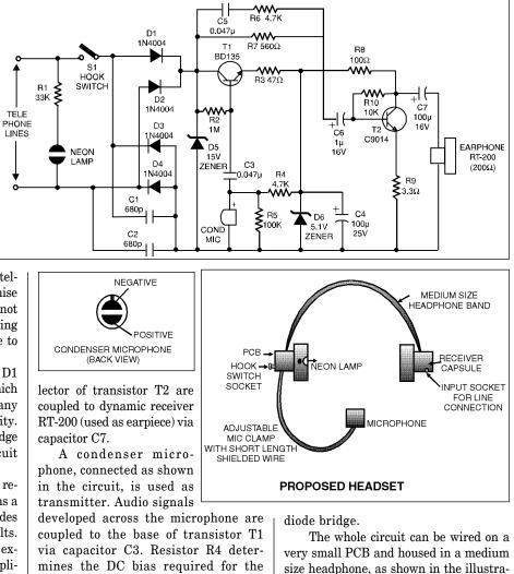
mines the DC bias required for the microphone. After amplification by transistor T1, the audio signals are
