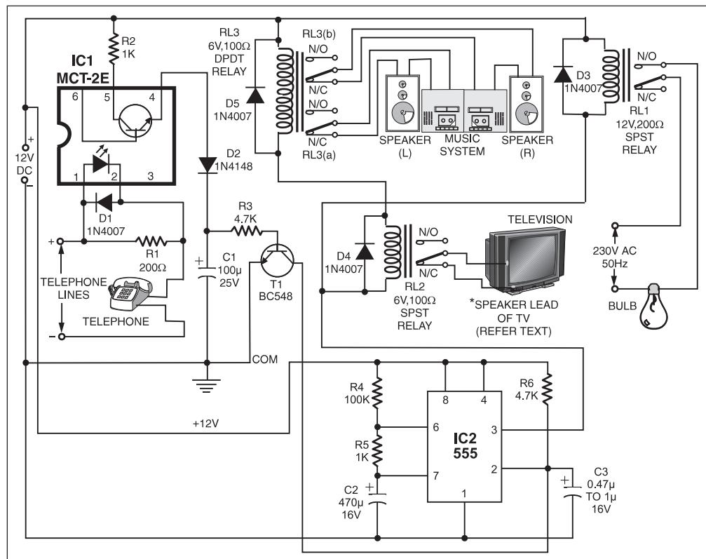
the in-built diode of IC1. After completion of call when handset is placed back on its cradle, the low-impedance path through handset is no more available and thus relays RL1 through RL3 are deactivated.
