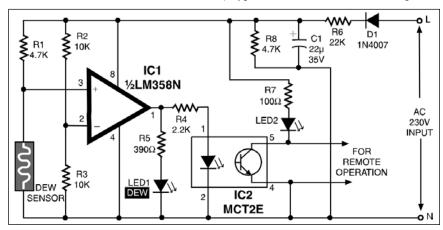
popular dual op-amp IC LM358N which is configured here as a comparator. (Note that only one half of the IC is used here.) Under normal conditions, resistance of the dew sensor is low (1 kilo-ohm or so) and thus the voltage at its non-inverting terminal (pin 3) is low compared to that at its inverting input (pin 2) terminal. The corresponding output of the comparator (at pin 1) is accordingly low and thus nothing happens in the circuit.
