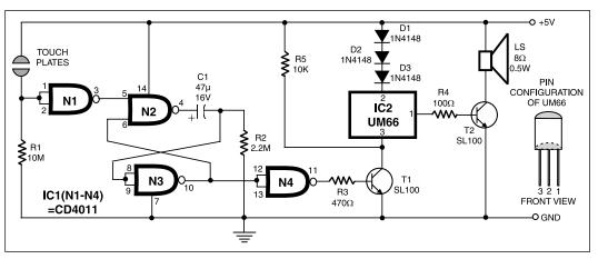
ing values of capacitor C1 and resistor R2. Three silicon diodes connected in series between pin 2 of UM66 IC and positive 5-volt rail keep voltage applied to pin2 of UM66 below 3.2 volts because of the drop of approximately 1.8 volts across them.
