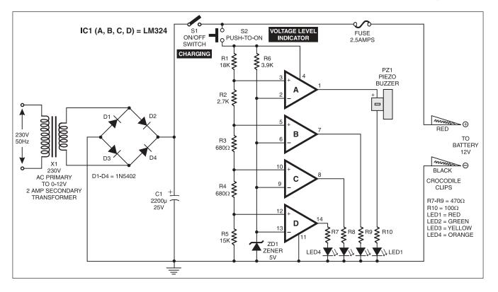
The different levels of battery voltages are indicated by LED1 through LED4. All the LEDs remain lit when the battery is fully charged (above 12.5V). The buzzer connected to the output of IC1 also sounds (when S2 is pressed with S1 kept open) as long as the voltage of battery is above 9.8V. If the voltage level goes below 9.8V, the buzzer goes off, which indicates that it's time to replace the battery. The status of LEDs for different battery voltages is shown in the table.
