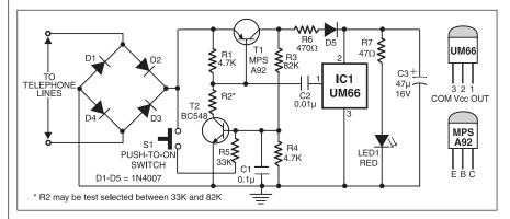
gets the supply and is activated. The music is coupled to the telephone lines via capacitor C2, resistor R1, and the bridge rectifier.
